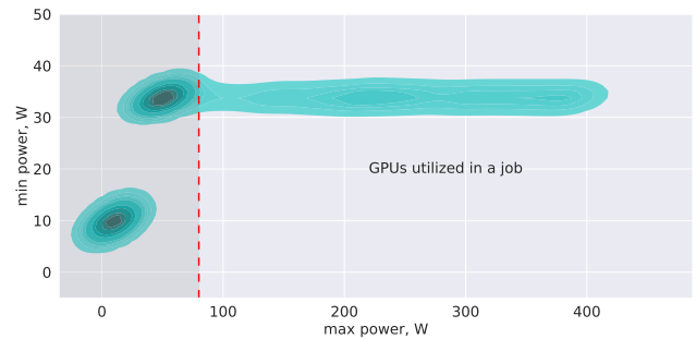
Figure 7: Distribution of GPU power consumption extrema in individual jobs. Dashed line at 80W shows the cut-off value to deem GPUs utilized by the job.
